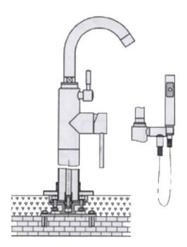
7. Connect the flexible hose (8) and handle shower (9) with the main body assembly (1), and place the shower handle (9) on the shower hook.
