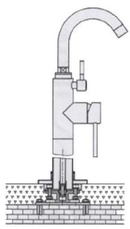
6. After installed the main body (1), install the out pipe unit (10) as shown on the above Fig.
